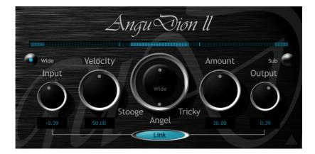
There is no Bypass on the AnguDion II. You must use the on/off button on the Pyramix plug-in container to compare dry and wet signal.
